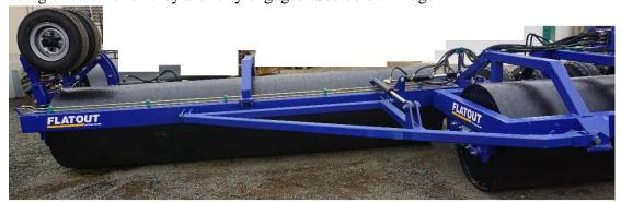
9. Before leaving the tractor, ensure that the park brake is applied and the engine is switched off. The a-frame lock must be secured in place using the safety lock located at the front of the center roller directly beside the a-frame lock pin in the working position.
